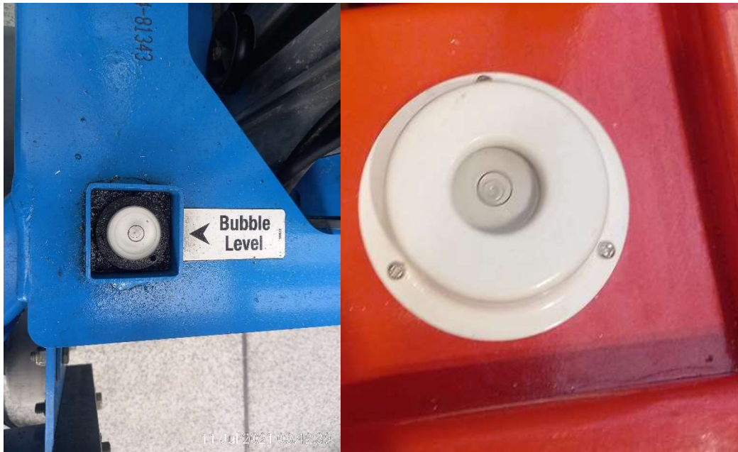
Photo 11 Water Pas Level Adalah Pengukur Kedataran & Stabilitas Alat Manlift Seperti Gelas Bening Yang Tertutup & Hanya Diisi Satu Titik Air Saja. Water Pass Level is A Measurement the Platness & the Stability of Manlift Such As a Transparant Closure Glass & Only Fill one Drop of Water in The Middle.
